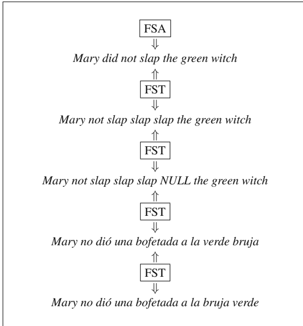
Fig. 2. The statistical machine translation model of [9] implemented with a cascade of standard finite-state transducers [8]. In this model, an observed Spanish sentence is “decoded” back into English through several layers of word substitution, insertion, deletion, and permutation
